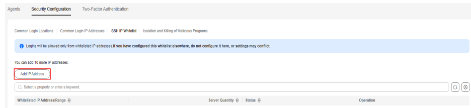
Figure 4-6 Configuring an IP address whitelist
